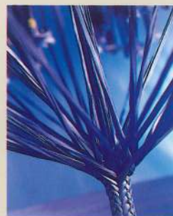
BRAIDING OF GLAND PACKING
