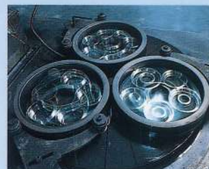
LAPPING OF MECHANICAL SEAL
